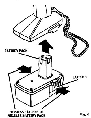
Make sure the latches on each side of your battery pack snap in place and battery pack is secured in drill before beginning operation.
